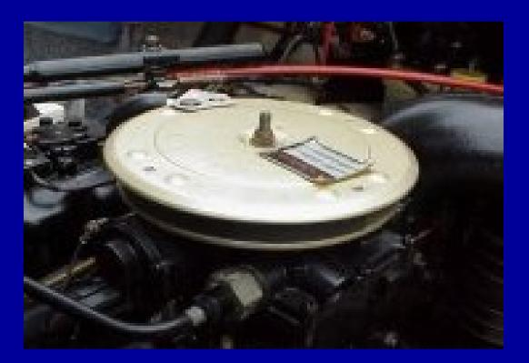
All gasoline powered inboard/outboard or inboard motor boats must be equipped with an approved backfire flame control device.
