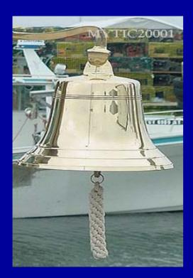
Boats 20 meters and over are required to carry a bell of 300 mm minimum diameter.
